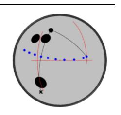
The "X" on the diagrams indicates the Preferred Spin Axis (PSA / Mass Bias) of the drilled ball, and the line that connects the PSA and PIN after drilling is referred to as the "Pin to Spin Line". The important feature of the "Pin to Spin Line" is that the ball revs up when the migrating axis crosses this line so the sooner the migrating axis crosses the "Pin to Spin Line".
