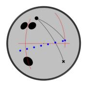
The "X" on the diagrams indicates the Preferred Spin Axis (PSA / Mass Bias) of the drilled ball, and the line that connects the PSA and PIN after drilling is referred to as the "Pin to Spin Line". The important feature of the "Pin to Spin Line" is that the ball revs up when the migrating axis crosses this line so the sooner the migrating axis crosses the "Pin to Spin Line", the sooner the ball revs up.
